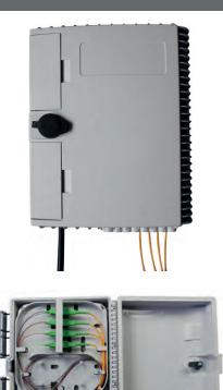
Accommodate 1x8-1x16PLC Splitter Anti-UV (Ultra Violet) Waterproof Up to 16 FTTH Drops 2 inlet ports, 16 outlet ports Accommodate SC /LC Adaptor It is applicable for wall-mounted, indoor or outdoor Max capacity(F): 16 315x236x108.5 2 cable ports (for cables with max 16 mm) 16 drop cable ports 16 Splices 1x8, 1x16 PLC Splitter 16 SC Simplex Adaptors
