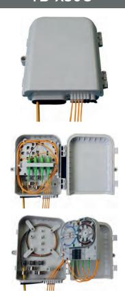
Accommodate 1x4-1x8PLC Splitter Anti-UV(Ultra Violet) Up to 12 FTTH Drops 3 inlet ports, 12 outlet ports Accommodate SC /LC Adaptor It is applicable for wall-mounted indoor or outdoor Max capacity(F):12 ROHS compliance 233x204x77 3 cable ports (for cables with max 14 mm) 12 drop cables ports 12 Splices 1x4. 1x8 PLC Splitter 12 SC Simplex Adaptors
