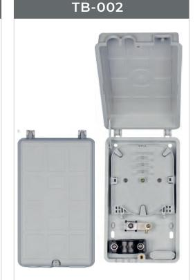
Light weight, small size, easy installation. Provide splice connection protection of fiber cable and pigtail Made of engineering plastic material, which has mechanical strength reliable and long lasting, Slide-N-Lock fiber optic splice tray with its opening angle above 90°C Therefore it is easy for installation and maintenance 197x110x44 mm Number of entry exit ports:2 Number of Splice Trays:2 Max. Fiber Count: 24 Max. Number of Pigtails :12
