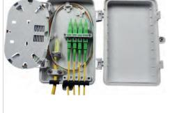
Can hold 1x4 PLC splitter Up to 4 drop cable Up to 4 SC adaptors 1 inlet port( for cables with max diameter 8mm) 4 outlet ports Wall mounting Protection class: IP 55 ROHS compliance Dimensions:210mmx140mmx40mm Re-usable, UV resistant and weather proof ROHS compliance, IP55
