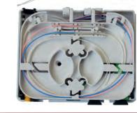
Ergonomically design, compact design Ability to allow cables to enter from rear or bottom of the unit Removable cover for easy access Indoor use for Wall mounted unit used for small and large business premises Easily re-enter with a minimum of tools, saves time and cost, Can be used for Blown Tube cable or common cables ROHS compliance 108.5x85x27mm Can hold 2 SC simplex adaptor or 2 LC duplex adaptor Three (3) cable ports, each port for one cable with maximum diameter Ø 10 mm
