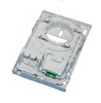
Can be used flush mount or surface mount Compatible with almost any standard electricity box; Removable fiber organizer system facilitates an easy installation Guaranteed minimum bending radius of 20mm Splice-through function allows moving the FO Access point to any other point in the premise Environmental friendly materials, low smoke zero halogen
