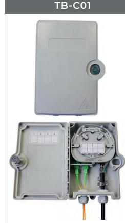
Construction-lightweight plastic offers strength and resistance to chemical and U.V attack Wall mounting or pole mounting IP55 207x152x51.7 Number of entry exit ports : 2 cable ports (for cables with max diameter 12mm) Max. Nm. of Adaptors: 4 SC Simplex Adaptors PLC Splitter: 1x4 Splitter
