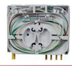
Very compact enclosure with dimensions Window cuts as small as 50mm possible with specific cable constructions such as the Mini-breakout cable Free breathing enclosure for indoor use Front accessible Wrap around riser cable installation Not required to cut loop-through fibers from riser cable Compatible with mechanical splice, heat shrink protectors in the same splice holder 108.5x85x27 mm 4 Splices Can hold 4 LC connectors or 2 SC connectors
