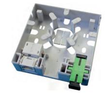
Ability to allow cables to enter from both sides of the unit Removable cover for easy access Compact, low profile, wall mounted unit used for small and large business premises 86x86x30.5 mm 1 SC Simplex Adaptors, 1 RJ45 and 1 RJ11 Number of input cable ports: 4 Maximum Capacity: 2 fibers
